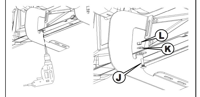
Drill two 3/16" holes through the long slot in the top of the brace.
