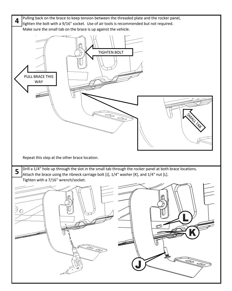
The next two steps are for the rear brace on the extended and crew cab pickup only. For the extended cab, measure back from the middle brace 20".
