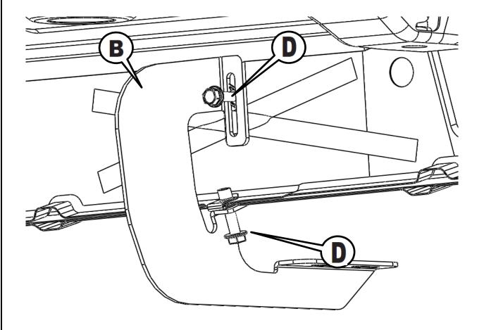
Tighten bolts with a 13mm Socket or wrench.
