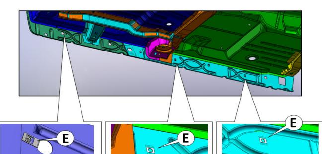
NOTE FOR 2007-2013: Your 2WD vehicle may not any preset fasteners in the hole patterns shown. If this is the case, use additional u-nuts (ITEM "E") to install in all locations as necessary.
