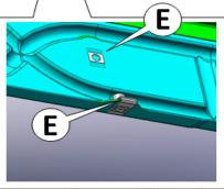
NOTE FOR 2007-2013: Your 2WD vehicle may not any preset fasteners in the hole patterns shown. If this is the case, use additional u-nuts (ITEM "E") to install in all locations as necessary.
