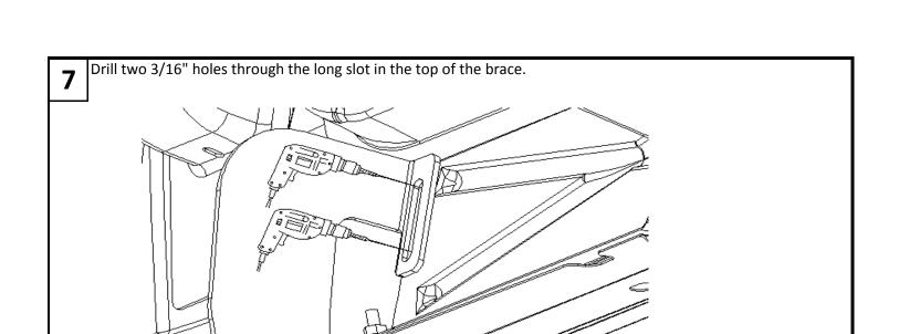
Attach the brace with two sheet metal screws [F] using a 3/8" wrench/socket.
