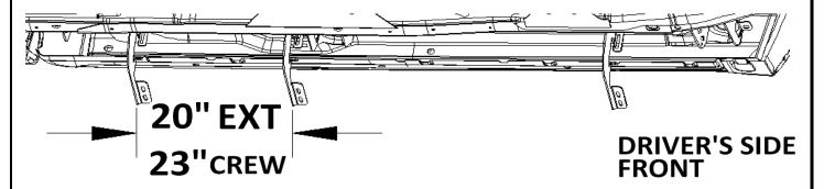
Hold the brace against the inner rocker panel and pinch weldl. Mark the slot in the small tab and drill a 1/4" hole through the rocker panel.
