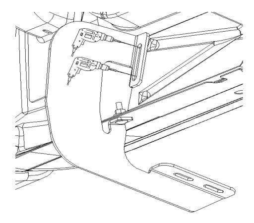
Attach the brace with two sheet metal screws [F] using a 3/8" wrench/socket.
